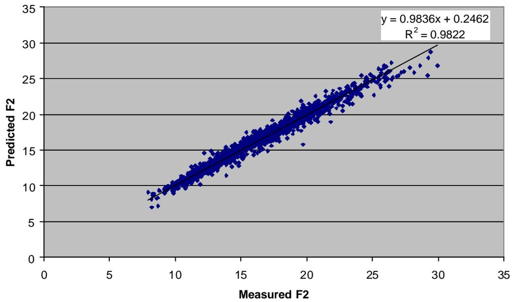
**Fig 2.** Predicted rolling force F2 [t] versus measured rolling force F2 [t] with a hybrid model (overall)
