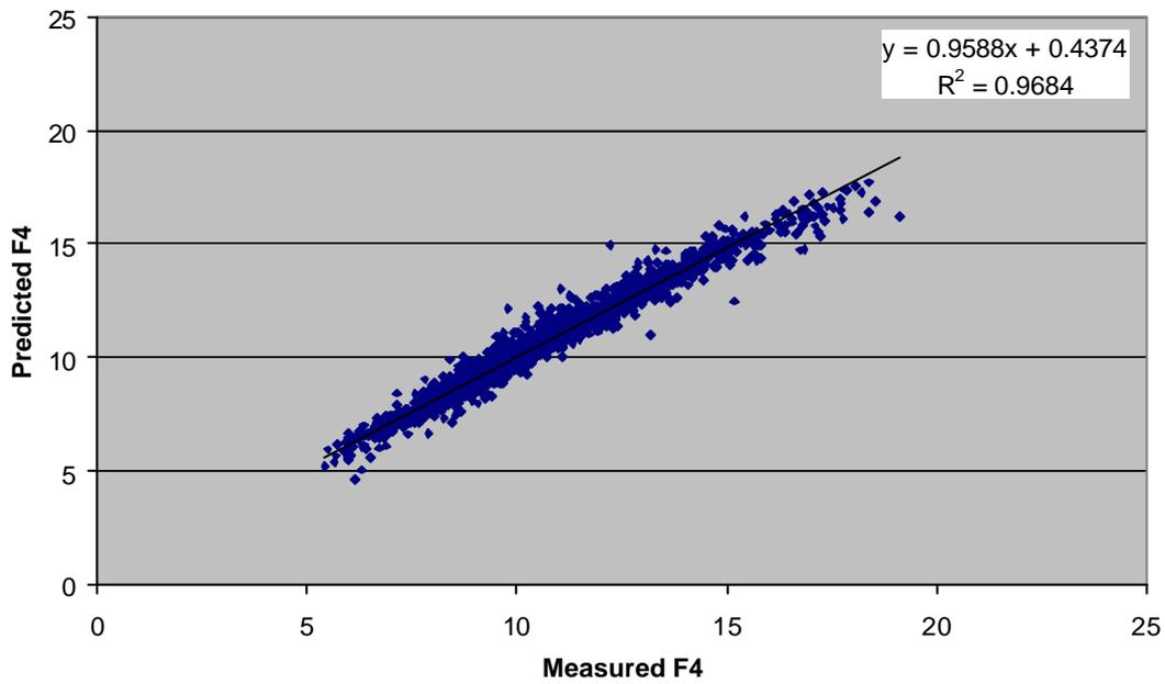
**Fig 4.** Predicted rolling force F4 [t] versus measured rolling force F4 [t] with a hybrid model (overall)
