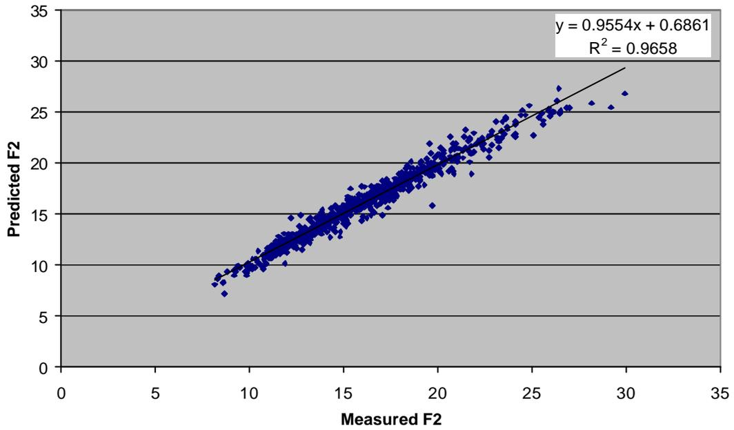
**Fig 7.** Predicted rolling force F2 [t] versus measured rolling force F2 [t] with a hybrid model (first bars)
