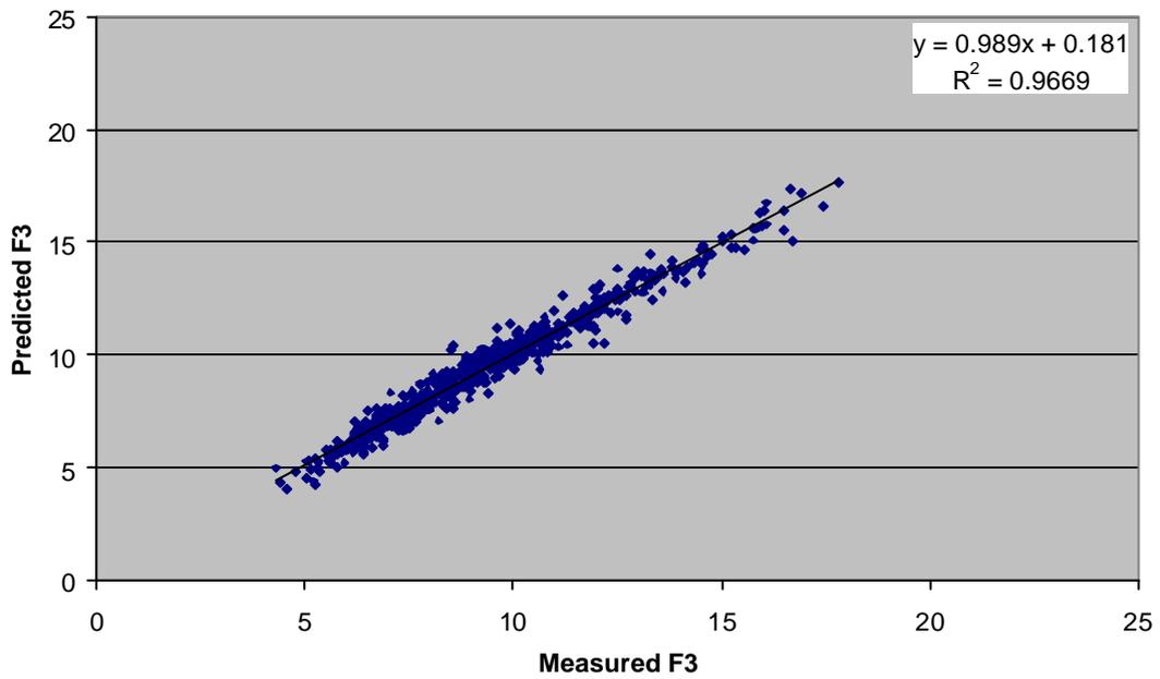
**Fig 8.** Predicted rolling force F3 [t] versus measured rolling force F3 [t] with a hybrid model (first bars)
