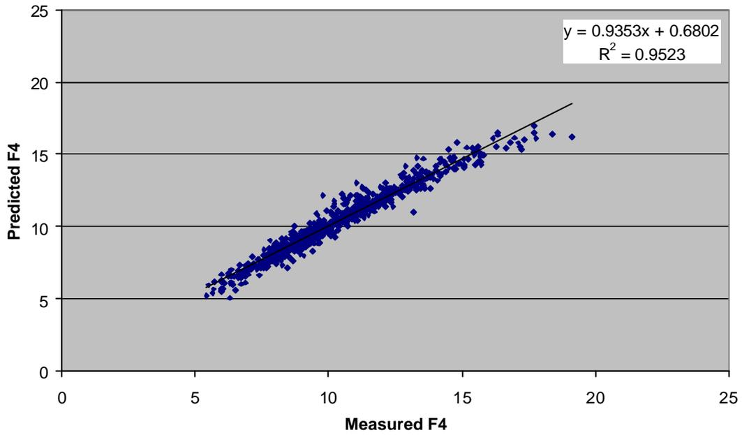
**Fig 9.** Predicted rolling force F4 [t] versus measured rolling force F4 [t] with a hybrid model (first bars)
