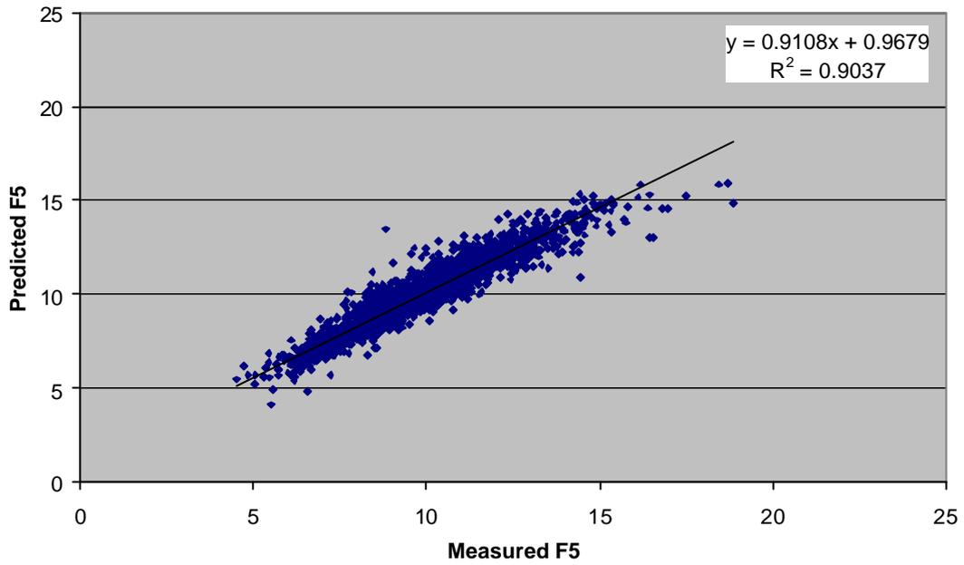
**Fig 5.** Predicted rolling force F5 [t] versus measured rolling force F5 [t] with a hybrid model (overall)
