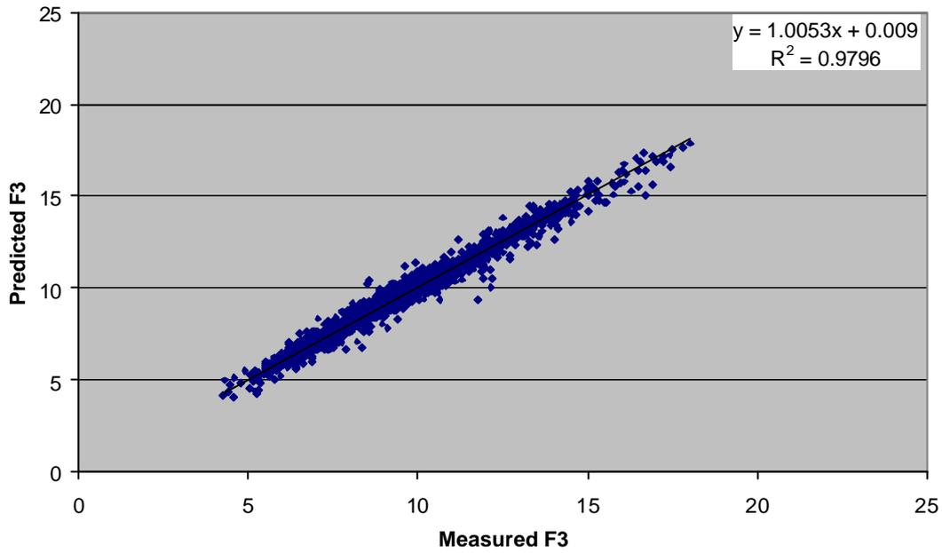
**Fig 3.** Predicted rolling force F3 [t] versus measured rolling force F3 [t] with a hybrid model (overall)
