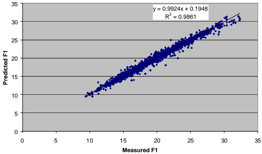
**Fig 1.** Predicted rolling force F1 [t] versus measured rolling force F1 [t] with a hybrid model (overall)
