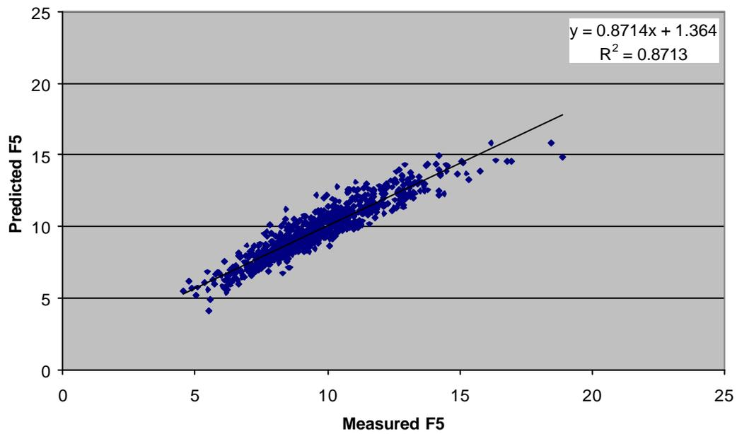
**Fig 10.** Predicted rolling force F5 [t] versus measured rolling force F5 [t] with a hybrid model (first bars)
