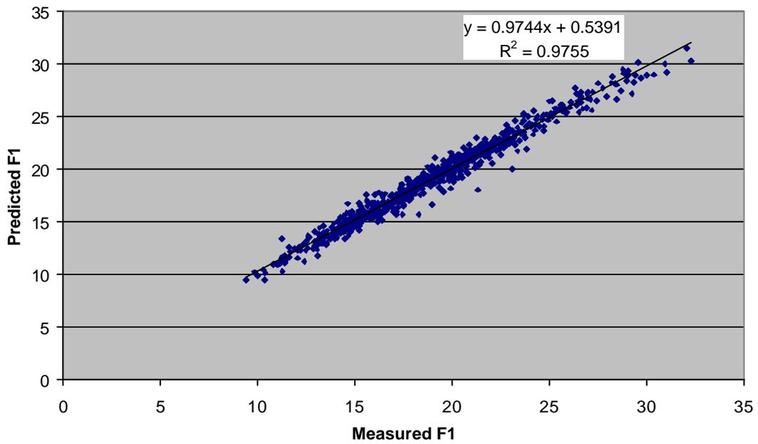
**Fig 6.** Predicted rolling force F1 [t] versus measured rolling force F1 [t] with a hybrid model (first bars)
